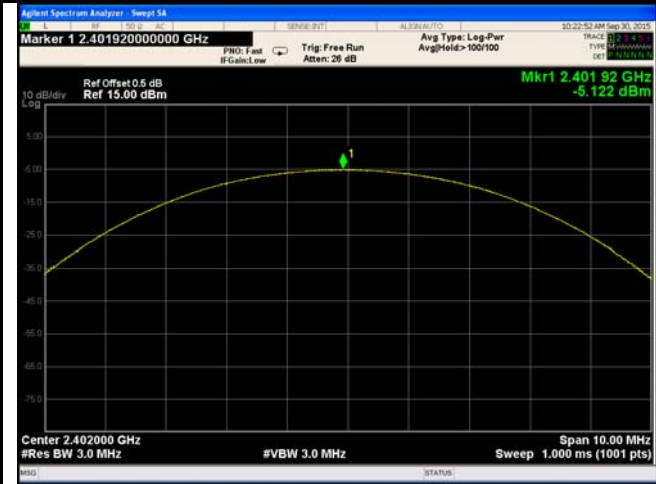
8DPSK Output power - Low CH 2402
