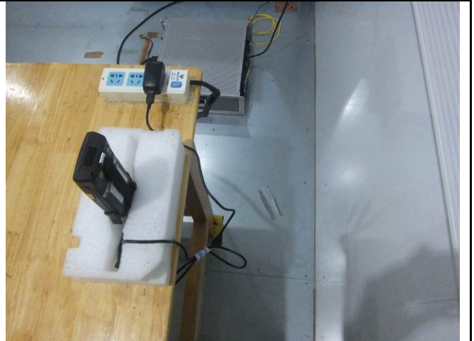
Conducted Emissions Test Setup Side View
