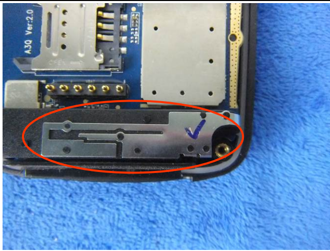
GSM/PCS/UMTS-FDD Antenna View
