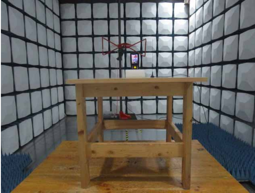
Radiated Emission View---Below 1GHz
