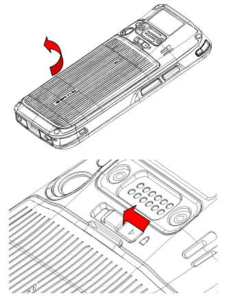
Figure 1-5 Installing and disassembling the battery cover
