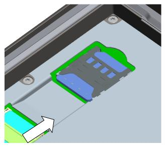
Figure 1-4 Inserting a SIM card
