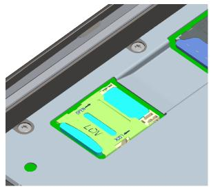
Figure 1-3 Inserting an SD card
