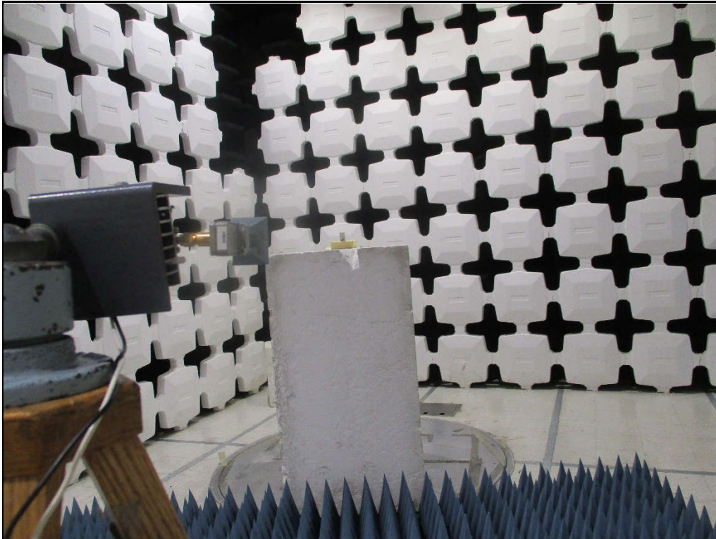
Test Setup for Spurious Radiated Emissions, Above 18GHz, Switch-B – Antenna Polarization Horizontal
