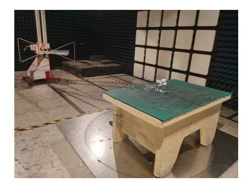
Spurious Emission Test Setup (Above 1GHz)
