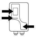
4. When the vehicle is fully charged, the Green light will stay solid, and the LCD screen will display a fully charged icon and 'Charging end' status. Your vehicle has a "dashboard gauge" that can verify full charge status, refer to the vehicle owner's manual to locate the gauge on your dashboard.
