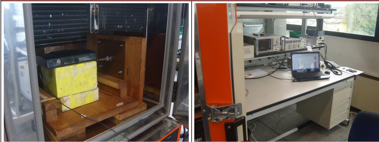
PHOTO N°6 SETUP FOR CONDUCTED MEASUREMENT
