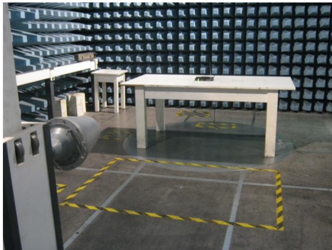
PHOTO N°3 SETUP FOR RADIATED MEASUREMENT >1GHz
