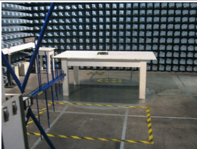
PHOTO N°2 SETUP FOR RADIATED MEASUREMENT <1GHz
