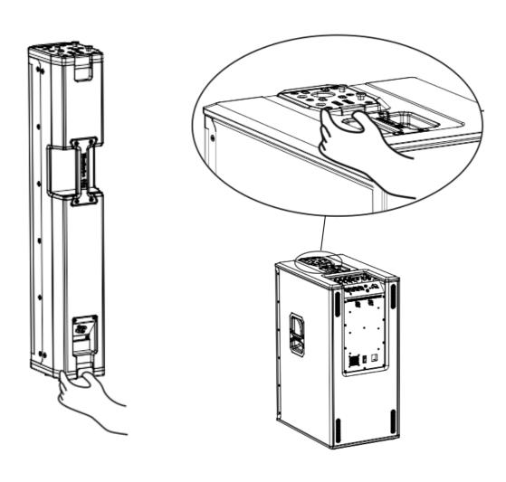
Align the locking systems and apply pressure to engage. If the assembly is correct, the safety levers move outwards (released position) with a "click".
