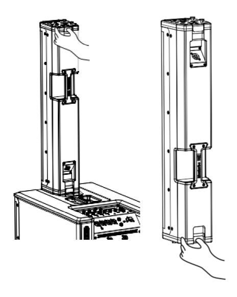
Place the second top on the first upside down, then align the blocking systems and apply pressure to engage. If the assembly is correct, the safety levers move outwards (released position) with a "click".
