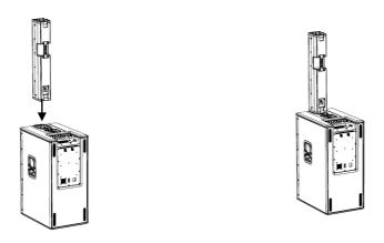
Push inwards the safety levers to arm the blocking systems of the two tops as shown.
