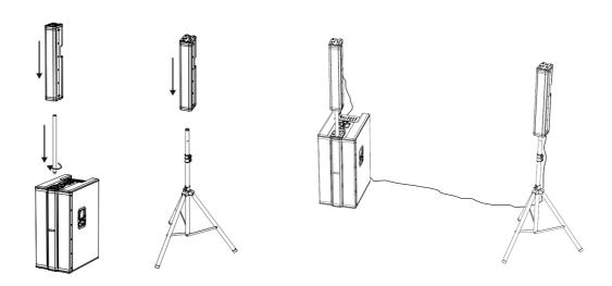
Connect the tops to the subwoofer using the speakON® supplied cables.
