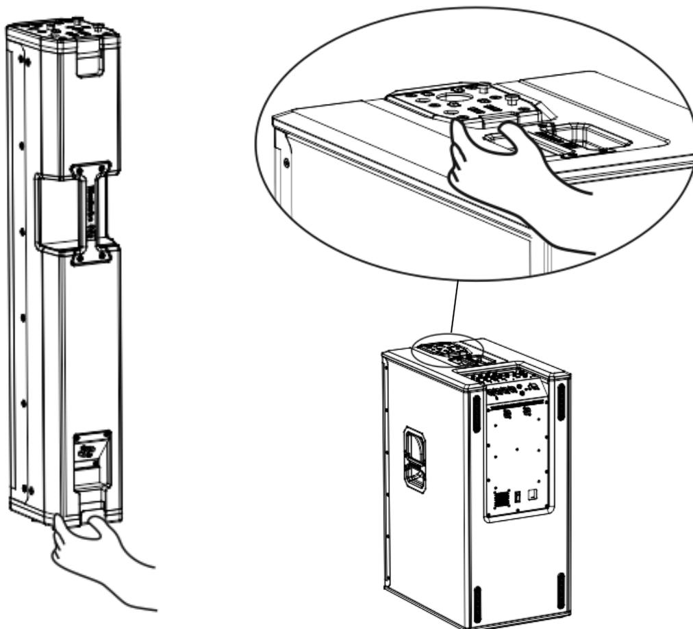
Align the locking systems and apply pressure to engage. If the assembly is correct, the safety levers move outwards (released position) with a “click”.
