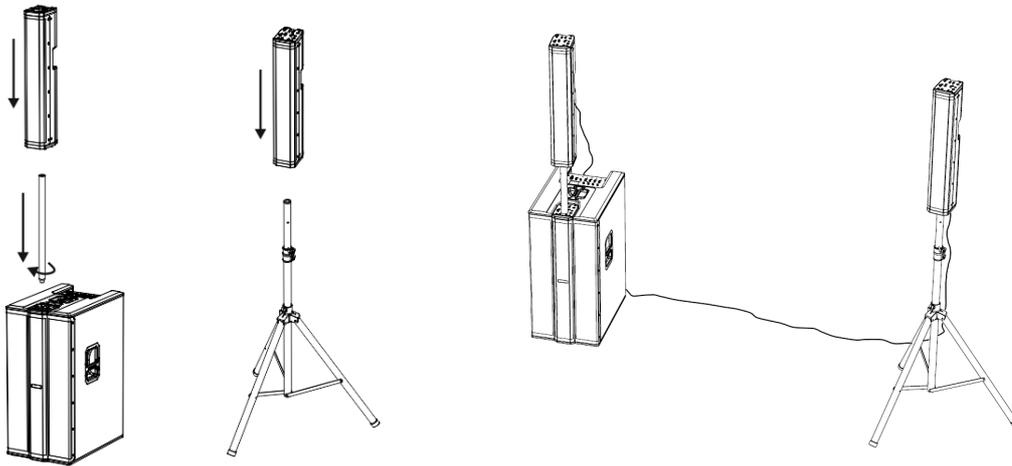
Connect the tops to the subwoofer using the speakON® supplied cables.
