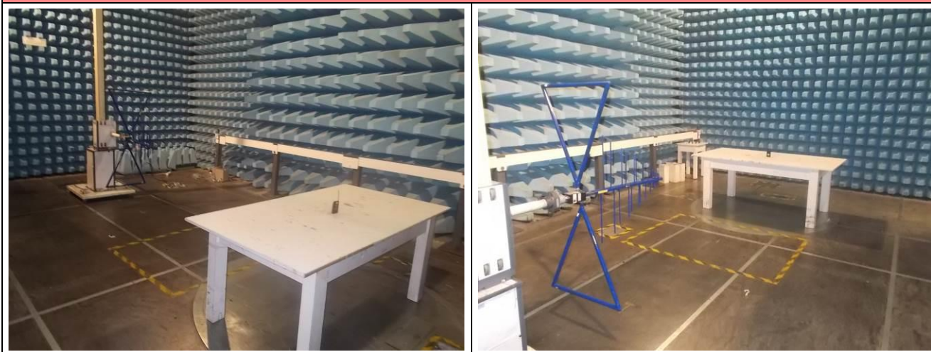
PHOTO N°2 SETUP FOR RADIATED MEASUREMENT <1GHz
