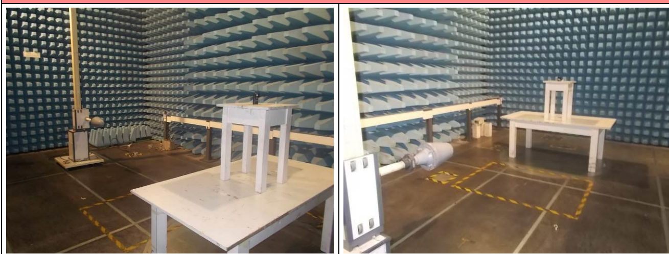
PHOTO N°3 SETUP FOR RADIATED MEASUREMENT >1GHz
