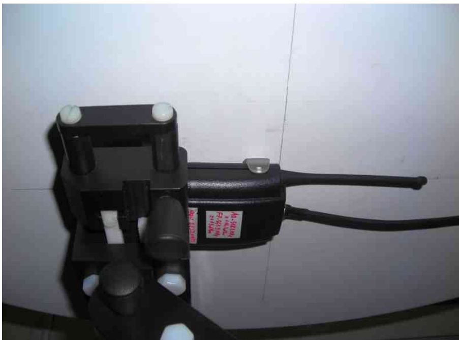
Figure 8 – Tested Device position: with the back side against the phantom
