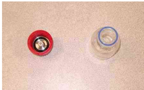
Figure 16 - Open coaxial probe with the bottle cap
