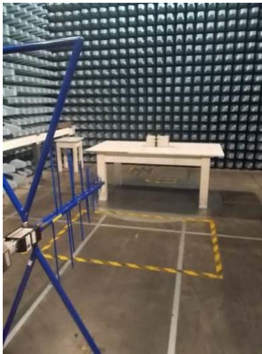
SETUP FOR RADIATED MEASUREMENT <1GHz
