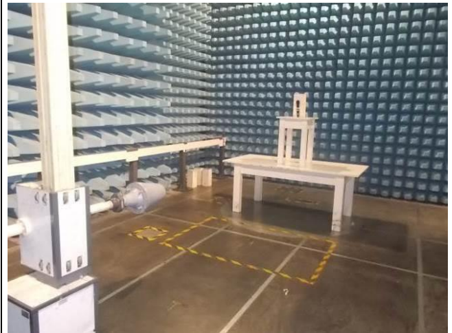
SETUP FOR RADIATED MEASUREMENT >1GHz
