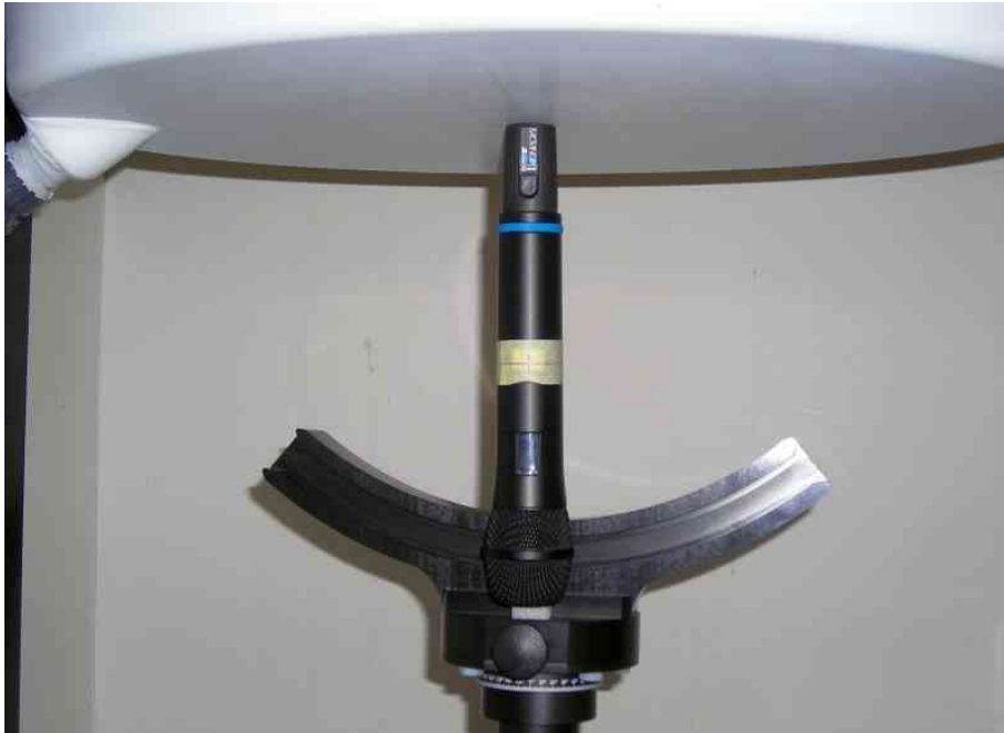
Figure 11 – Tested device position: with the Bottom against the phantom
