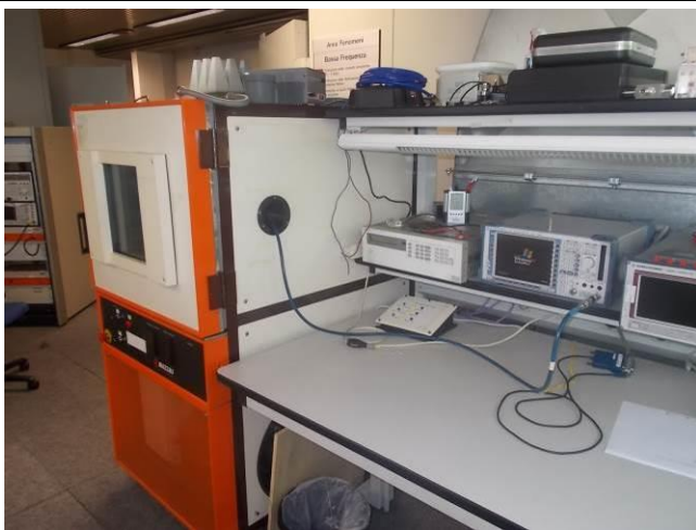
PHOTO N°4 SETUP FOR CONDUCTED MEASUREMENT
