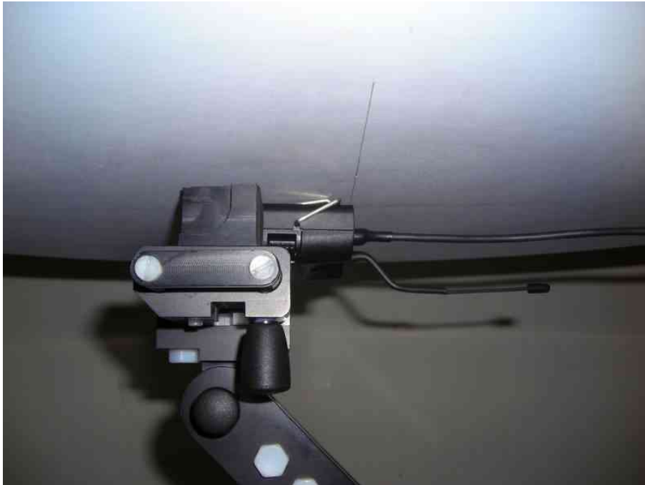
Figure 9 – Tested Device position: with the back side against the phantom (detail)
