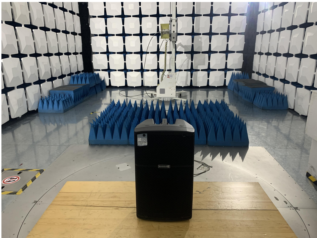
Above 1GHz for radiated emission test setup
