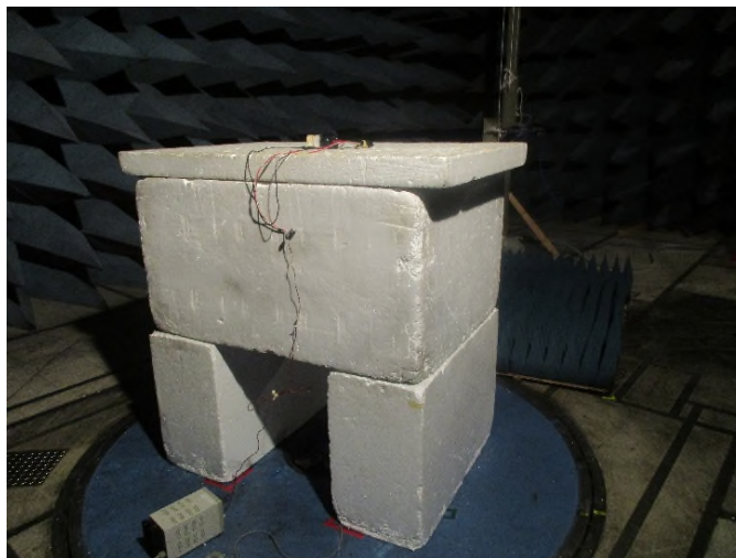
Figure 12: Radiated Emissions – above 1 GHz – Rear View – EUT on Side
