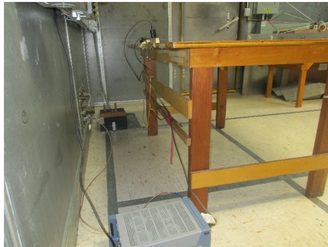
Figure 14: Conducted Emissions – Side View
