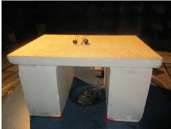
Figure 1: Radiated Emissions – below 1 GHz – Front View – EUT Flat
