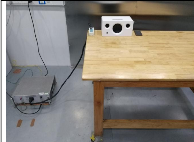
Conducted Emissions Test Setup Front View
