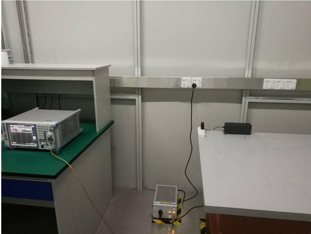
FCC RADIATED EMISSION TEST SETUP
