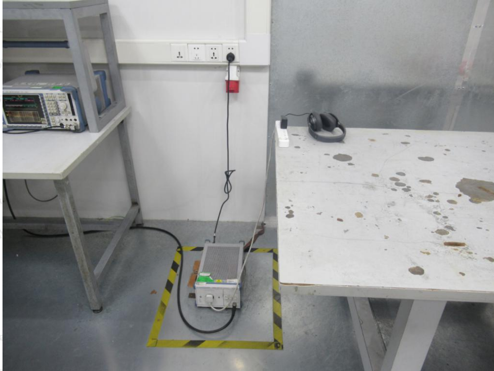
Photo of Conducted Emission Measurement
