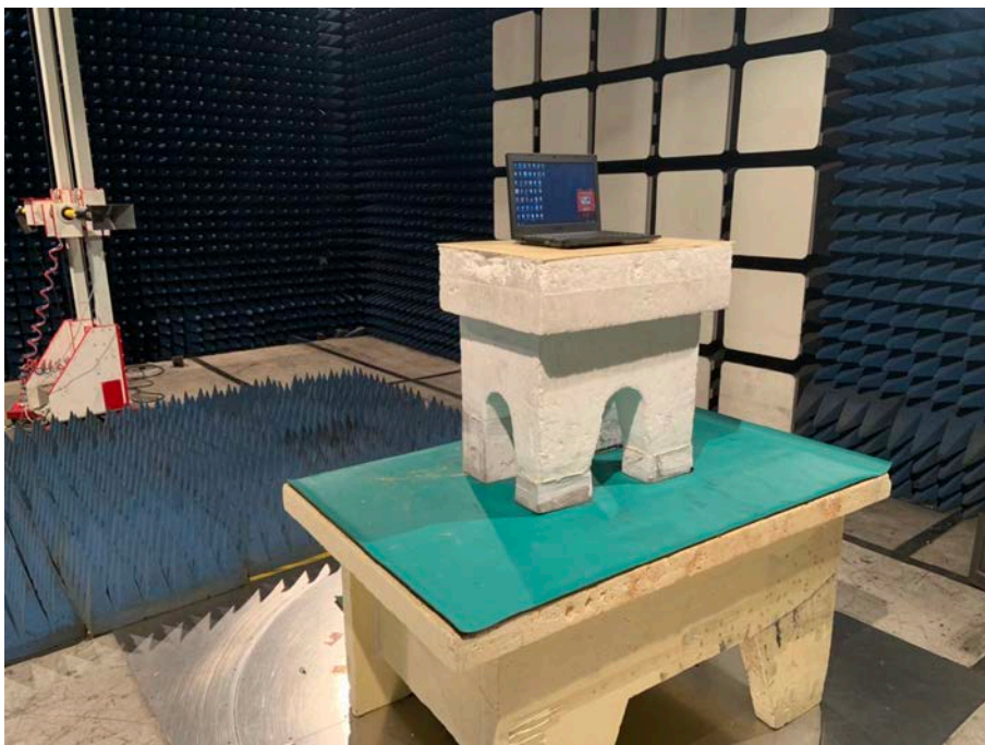
Spurious Emission Test Setup (Above 1GHz)
