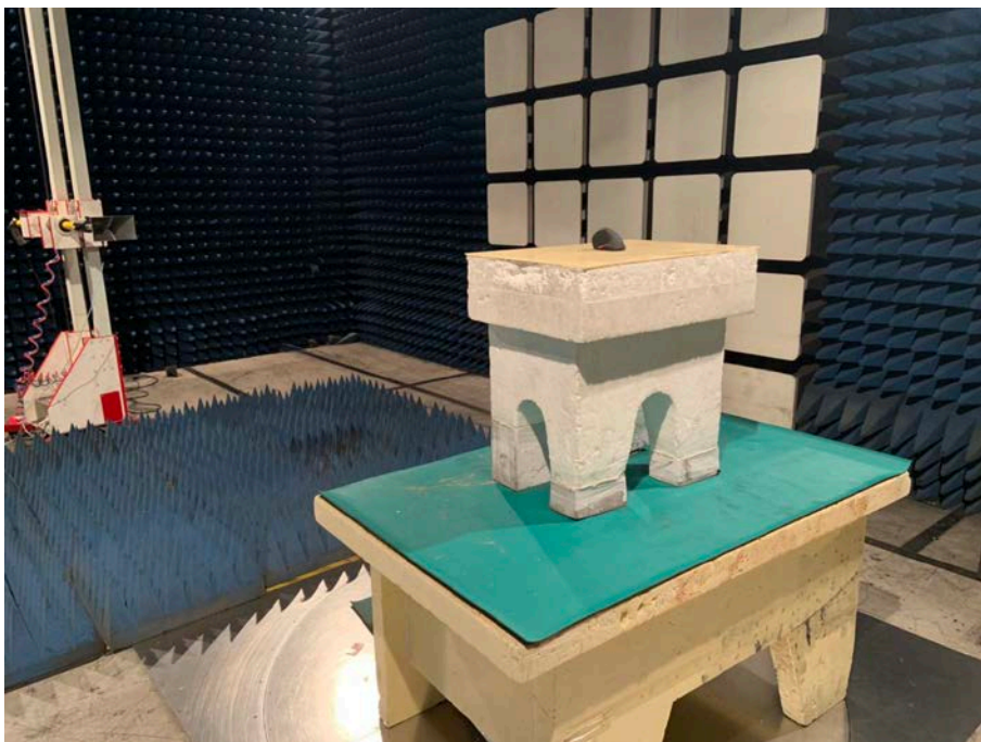
Spurious Emission Test Setup (Above 1GHz)
