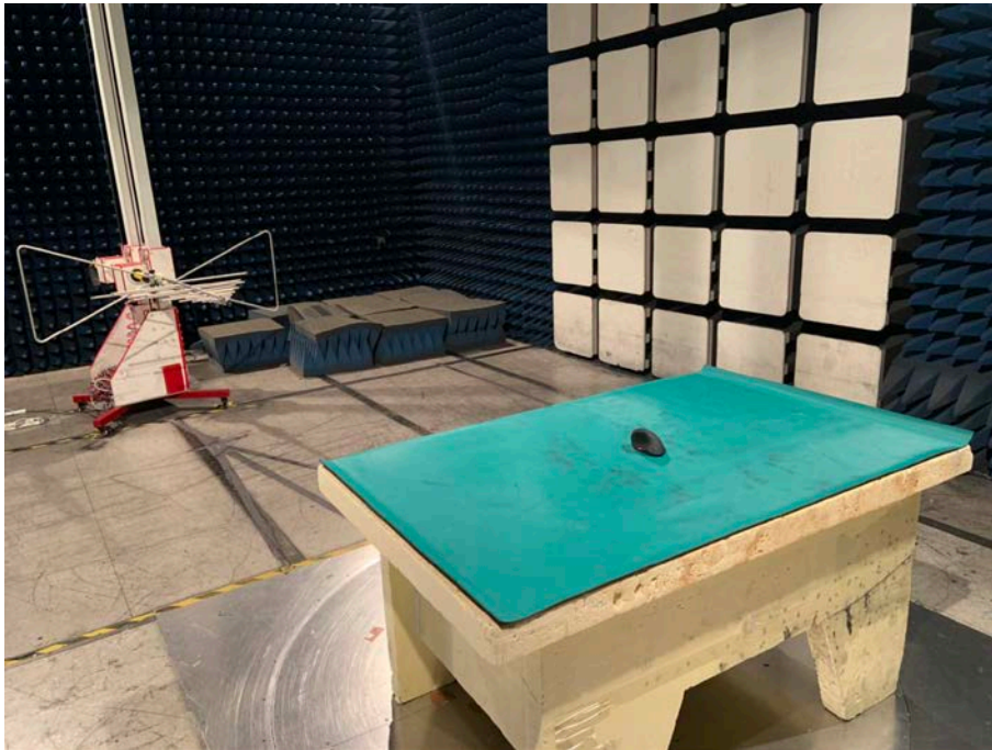
Spurious Emission Test Setup (Below 1GHz)
