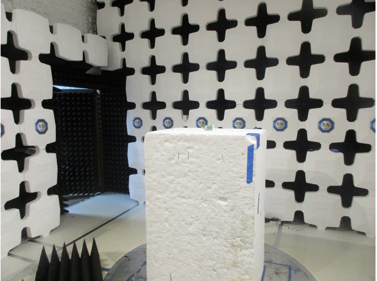
Figure 6: Radiated Emissions – Front View – above 1 GHz – EUT on Side (Band-Edge Measurements)
