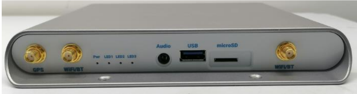
Figure 5: Wi-Fi/BT Antennae on SMA Connectors
