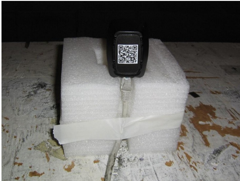
Radiated emissions test setup – EUT
