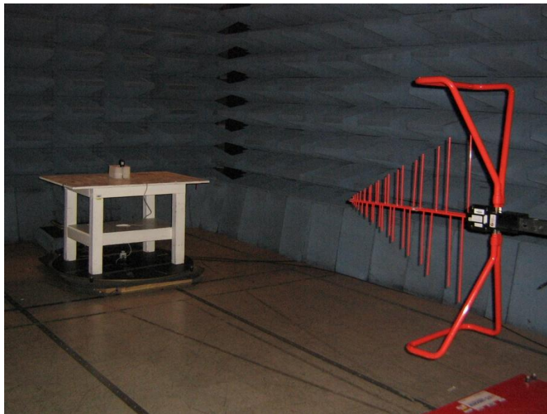
Radiated emissions test setup – 30MHz- 1GHz
