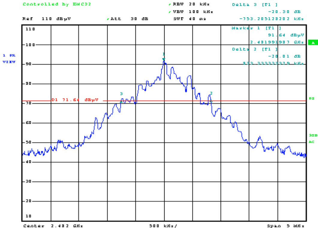
Plot 12: 20dB Bandwidth at HIGH Frequency – 1587 kHz
