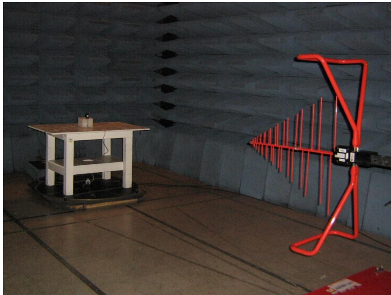
Radiated emissions test setup – 30MHz- 1GHz
