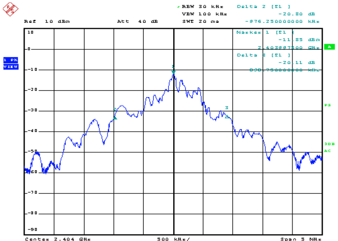
Plot 10: 20dB Bandwidth at LOW Frequency – 1875 kHz
