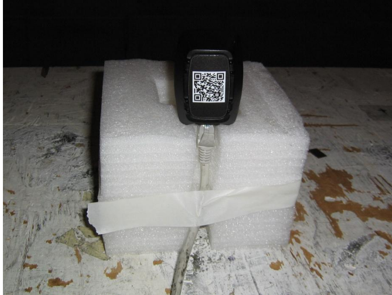
Radiated emissions test setup – EUT
