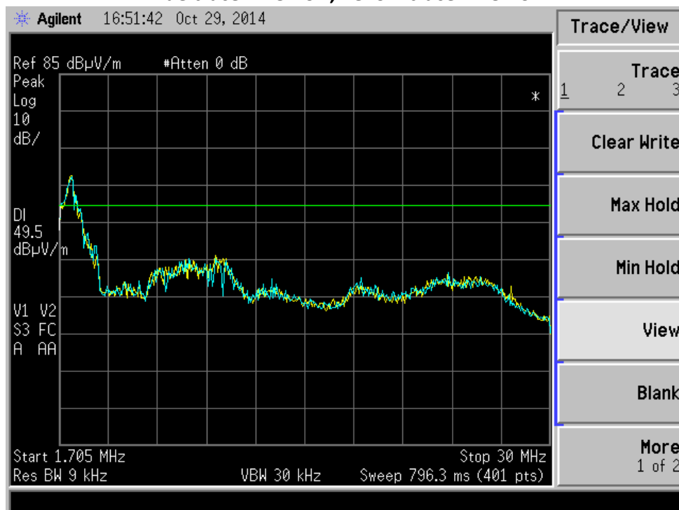
FIGURE 56: Active Loop, Vertical Polarization: 802.11 & BT Blue trace – EUT off, Yellow trace – EUT on
