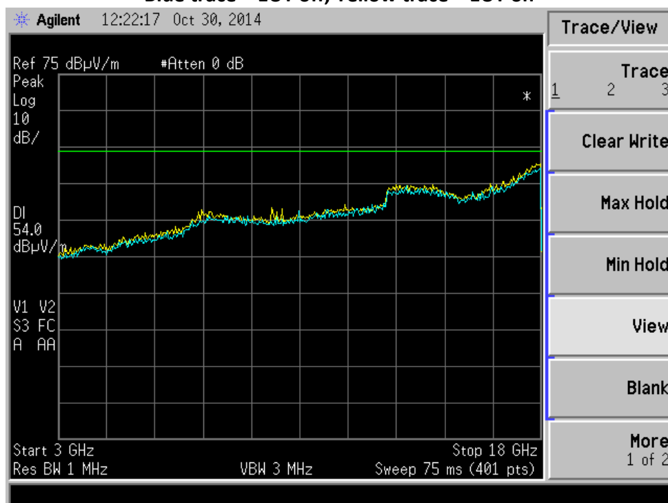
FIGURE 60: DRG Horn, Vertical Polarization: 802.11 & BT Blue trace – EUT off, Yellow trace – EUT on
