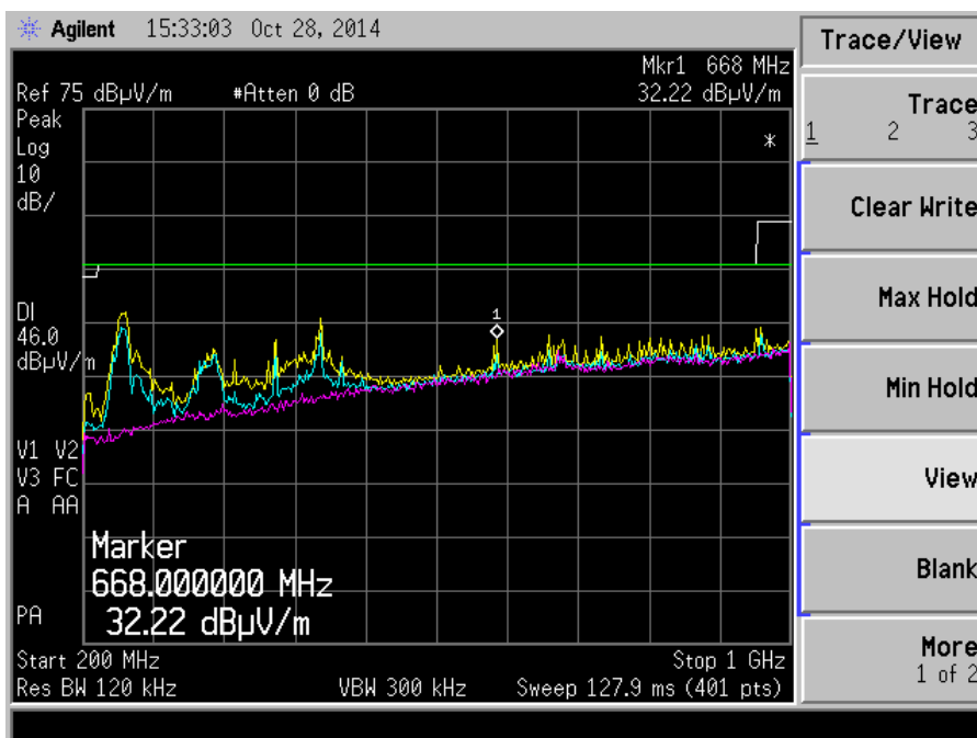
FIGURE 10: Radiated Emissions – Log-periodic, Horizontal Polarization Blue trace = EUT off, Yellow trace = EUT on, Magenta = chamber background
