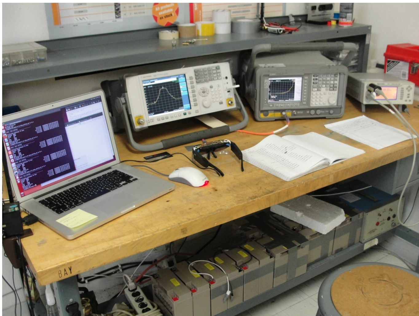
FIGURE 1: Conducted RF Test Setup
