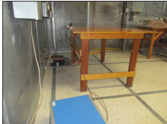
Figure 10: Power Line Conducted – Side View
