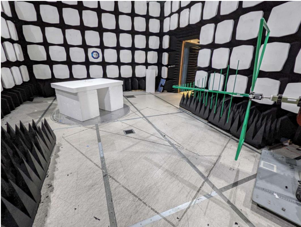
Figure 3: Equipment Under Test – Radiated Emissions <1GHz
