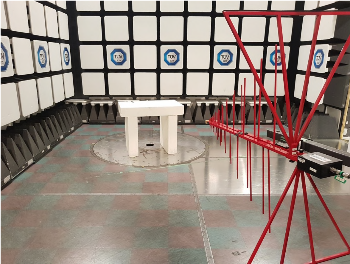
Figure 11 – Radiated Emissions Setup 30 MHz to 1 GHz
