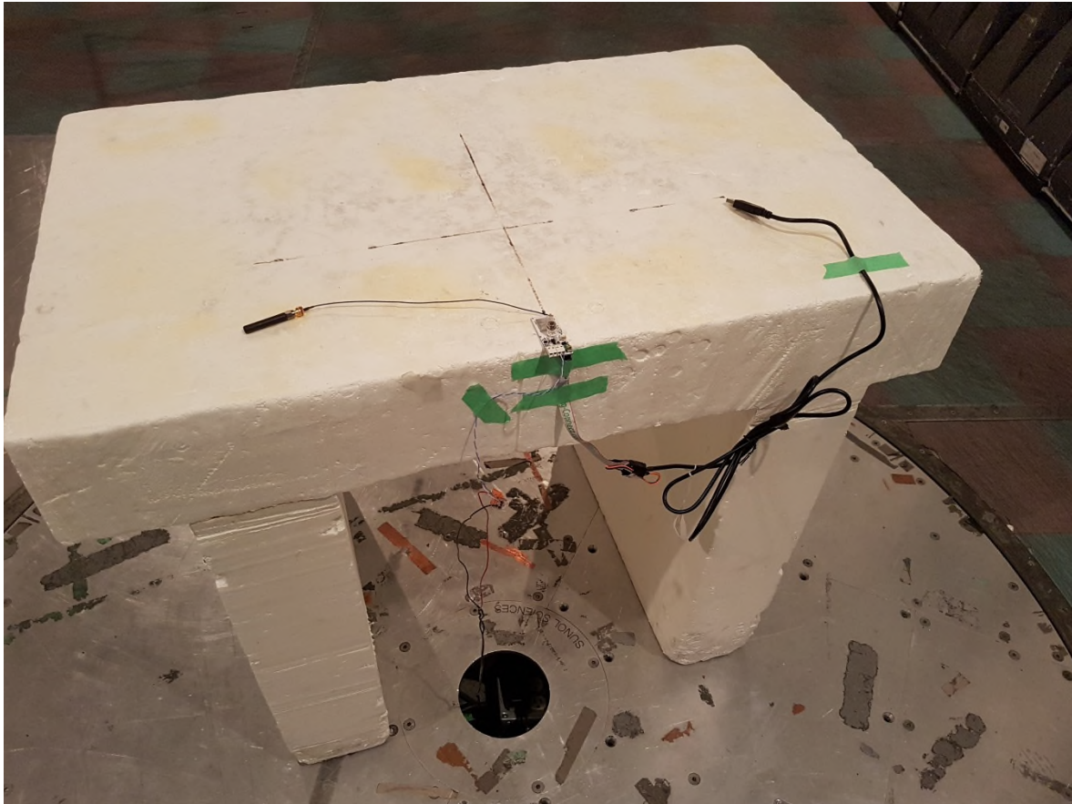
Figure 5 – Radiated Emissions Setup 915MHz EUT setup for max emissions Stubby Dual-Band Antenna
