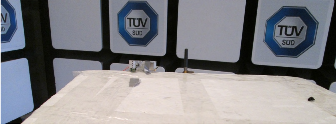
Figure 7 – Radiated Emissions Setup 2.4GHz EUT setup for max emissions Stubby Dual-Band Antenna
