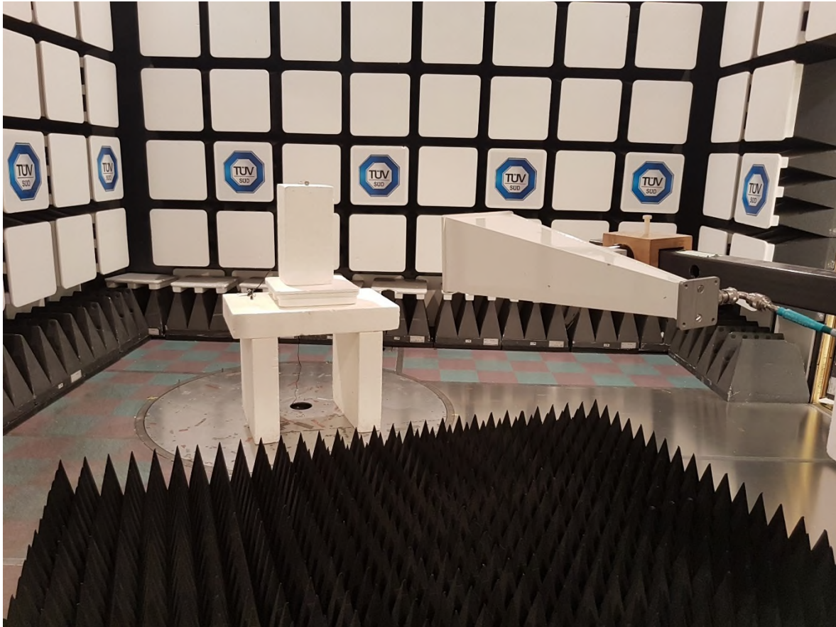
Figure 13 – Radiated Emissions Setup 4 GHz to 10 GHz (4 GHz to 18 GHz for colocation spurious scans)
