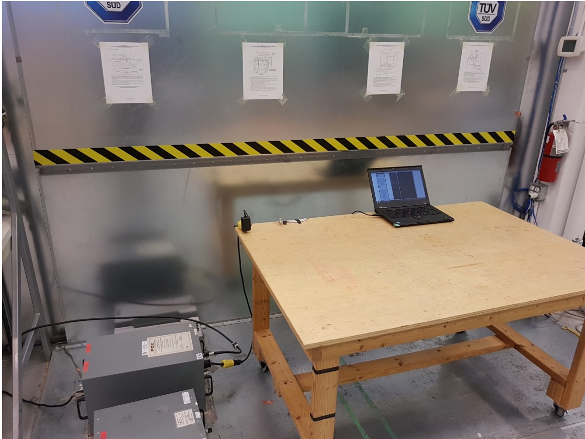
Figure 18 – Conducted Emissions Setup
