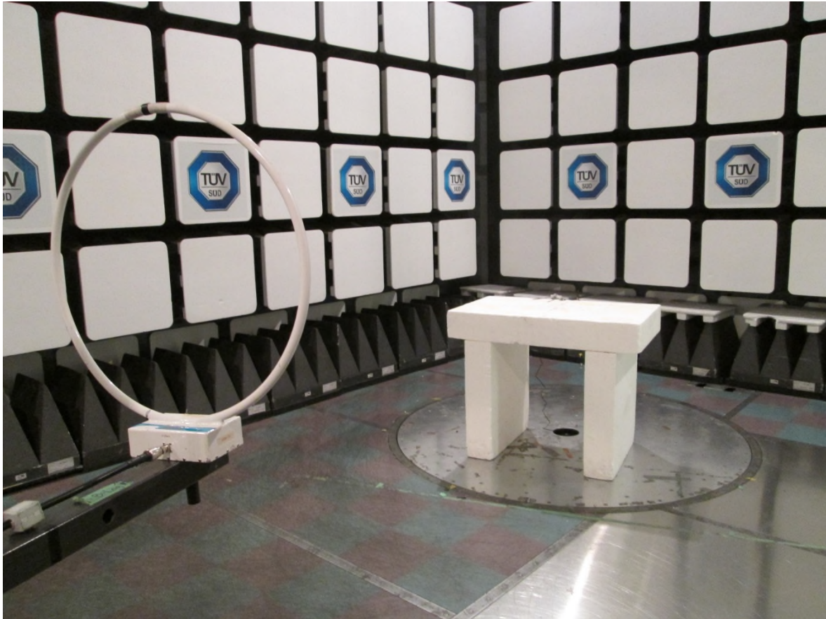
Figure 10 – Radiated Emissions Setup 9 kHz to 30 MHz
