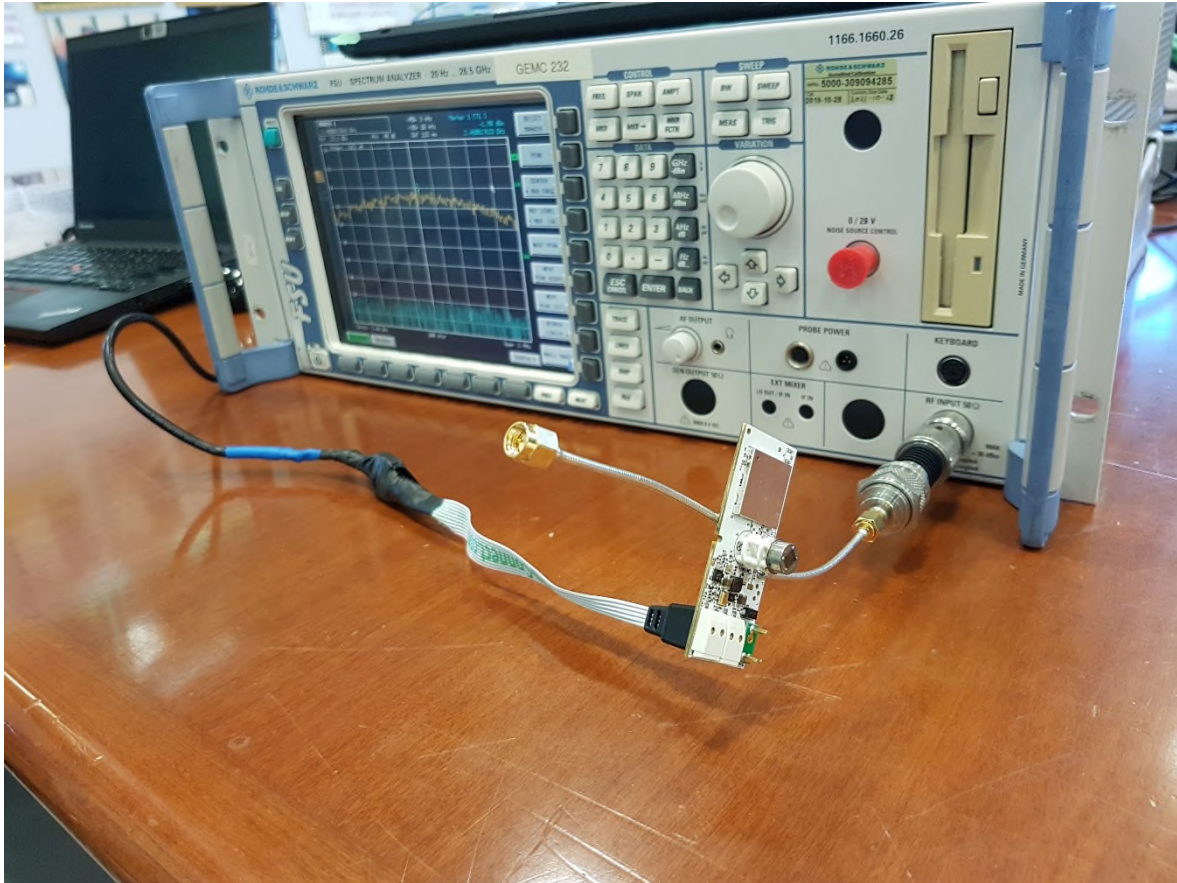
Figure 17 – Antenna Port Conducted Emissions Setup 2.4GHz Antenna Port
