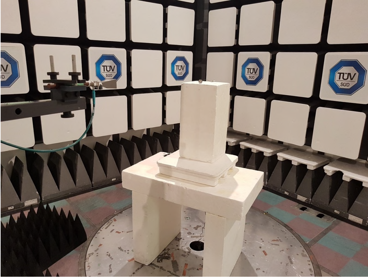
Figure 15 – Radiated Emissions Setup 18 GHz to 25 GHz
