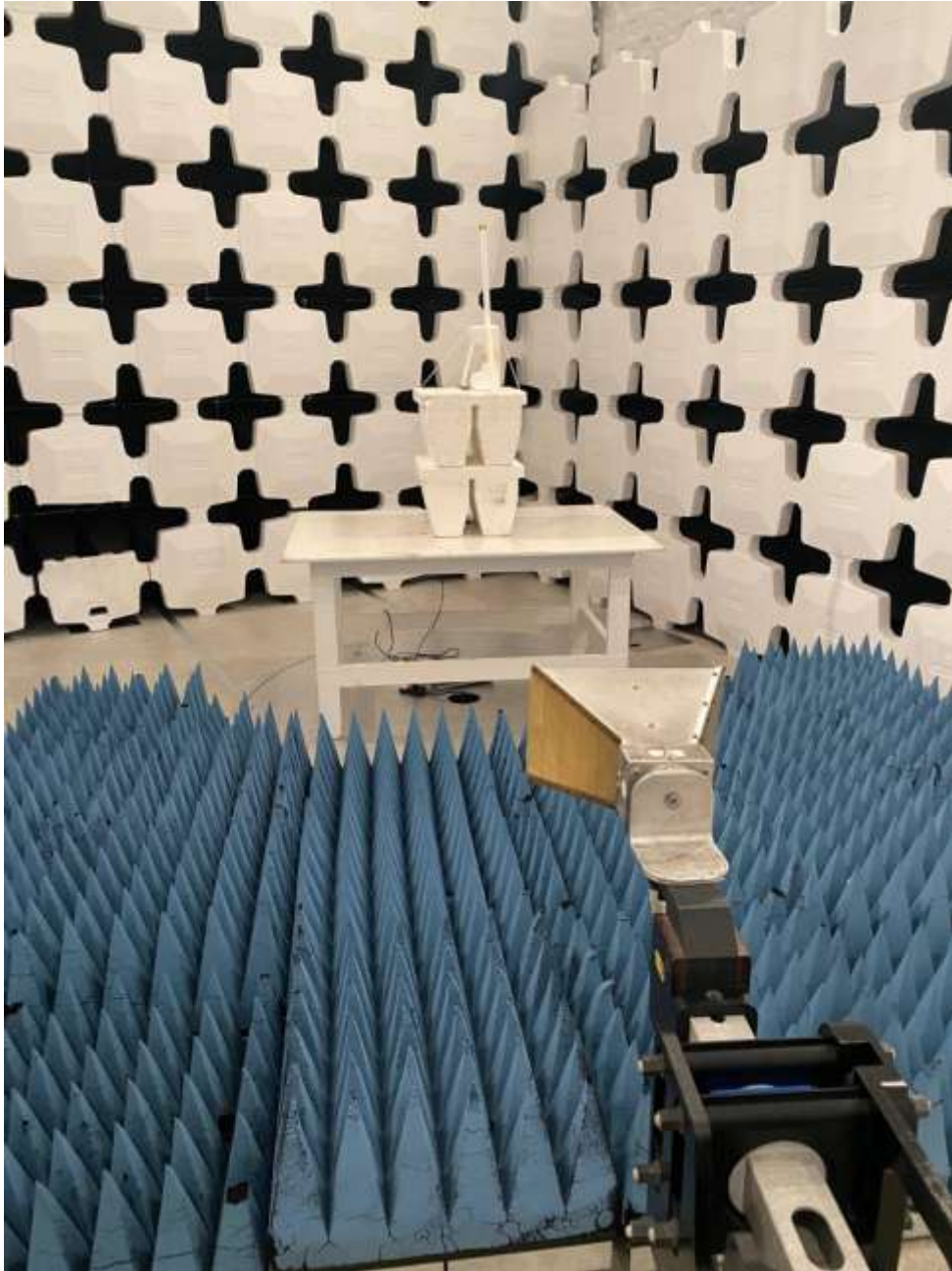
Figure 7. Radiated Emissions Test Configuration (Above 1000 MHz)
