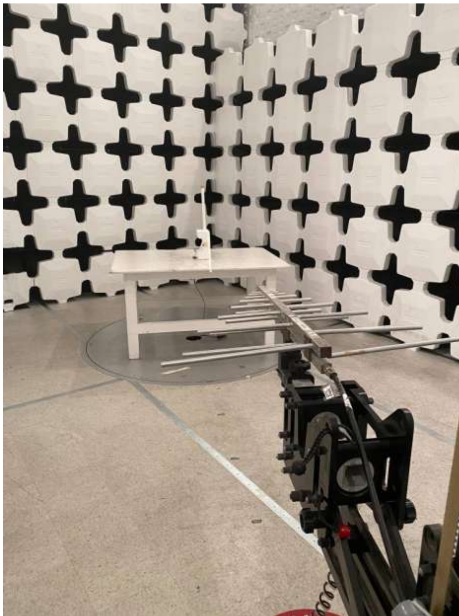
Figure 6. Radiated Emissions Test Configuration (200 MHz – 1000 MHz)
