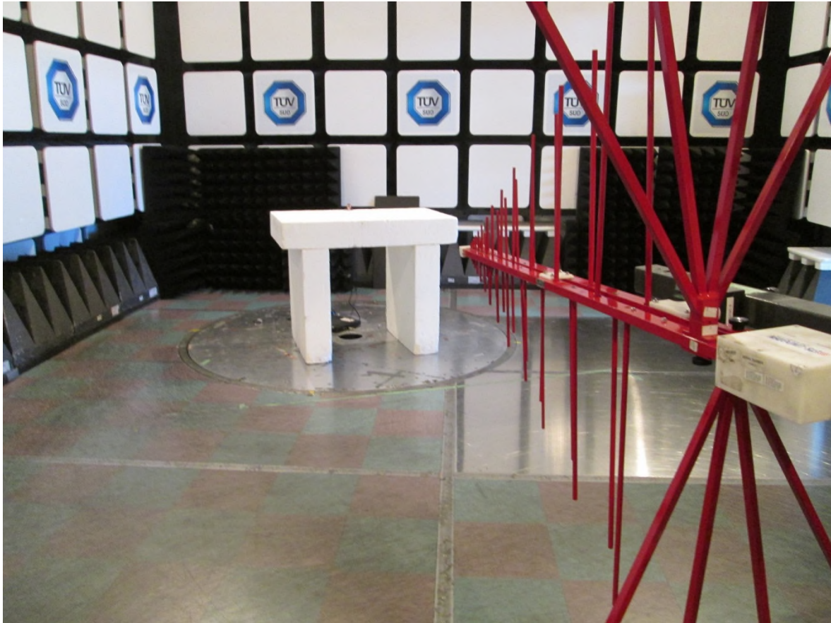
Figure 5 – Radiated Emissions Setup 30 MHz to 1 GHz
