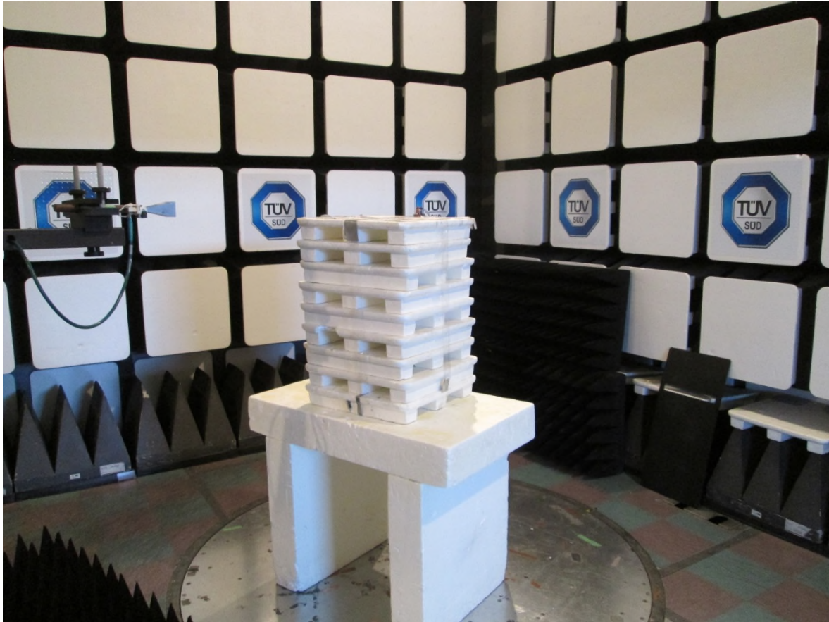
Figure 9 – Radiated Emissions Setup 18 GHz to 26.5 GHz
