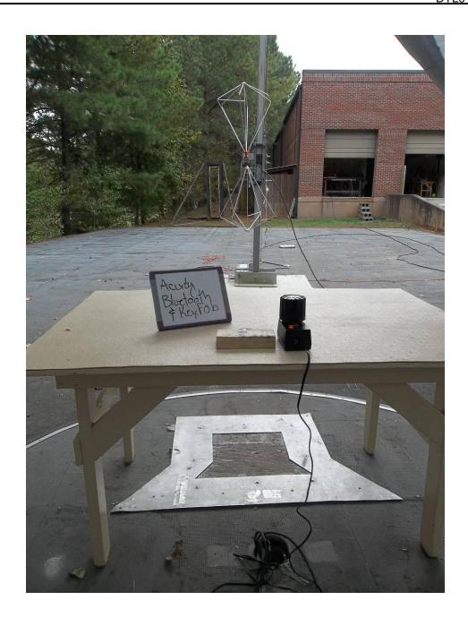
Figure 2. Radiated Emissions Test Setup, 30 MHz to 200 MHz, Back
