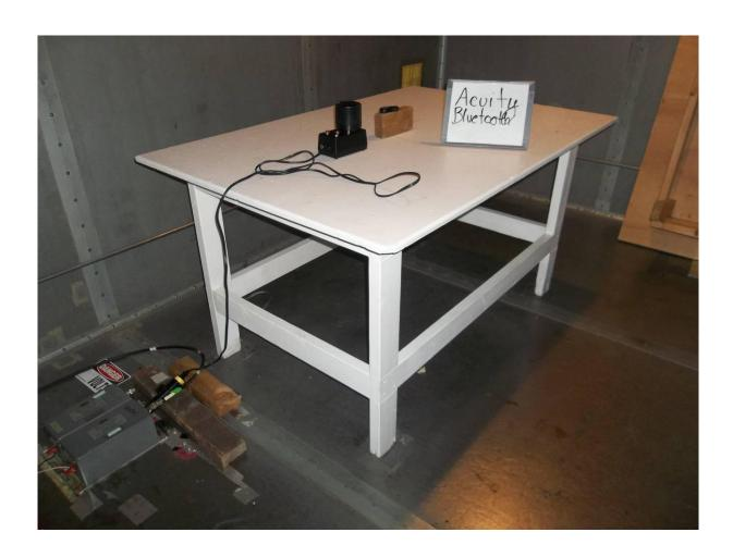
Figure 6. Conducted Emissions Test Setup
