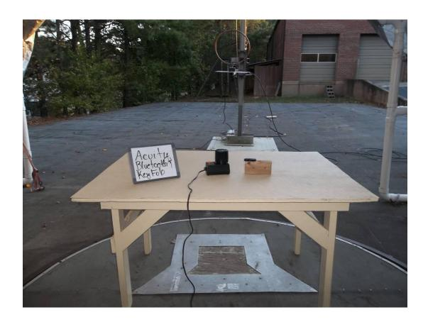
Figure 5. Radiated Emissions Test Setup, below 30 MHz, Back
