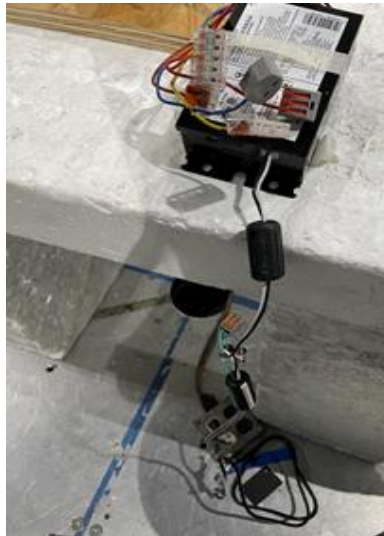
Figure 1.6-1: EUT setup pic with Fair-rite beads.
