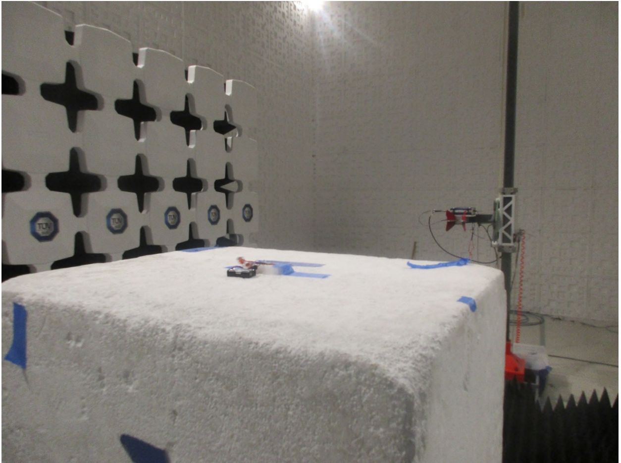
Figure 6: Radiated Emissions – Back View – PCB Trace Antenna
