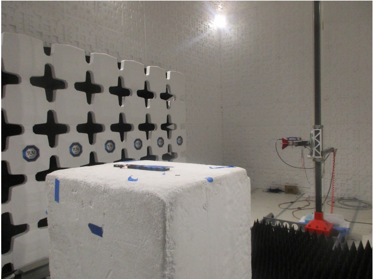
Figure 18: Radiated Emissions – Back View – External Flag Antenna
