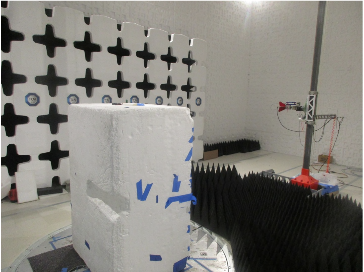
Figure 18: Radiated Emissions – Back View – Chip Antenna
