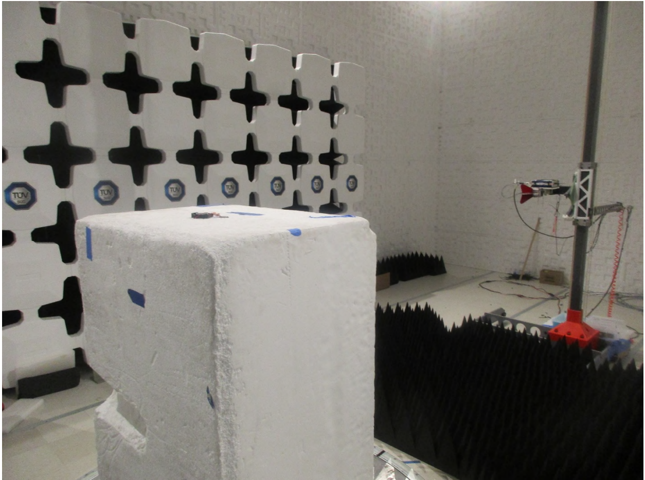
Figure 6: Radiated Emissions – Back View – PCB Trace Antenna
