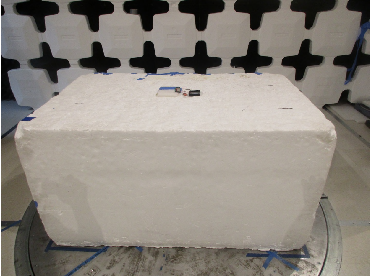
Figure 14: Radiated Emissions – Front View – Chip Antenna
