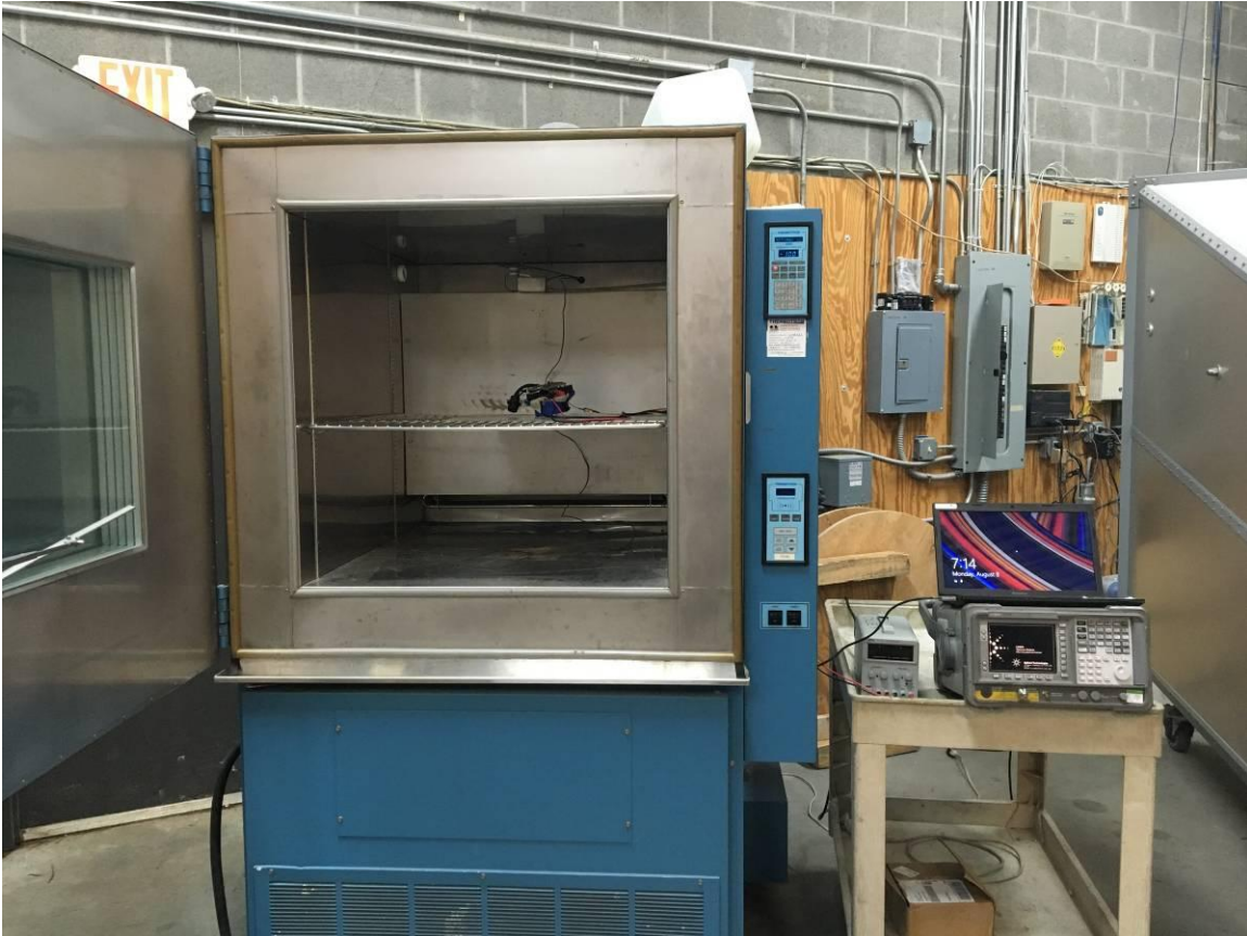
Figure 7. Extreme Temperature and Frequency Stability Test Setup
