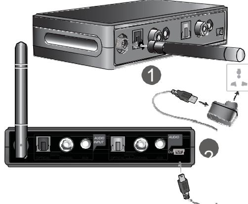
2. Connect audio cable and audio input/output
