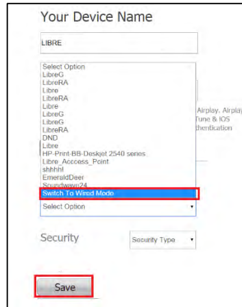
Figure 6.15-1: Switch to Wired Mode
