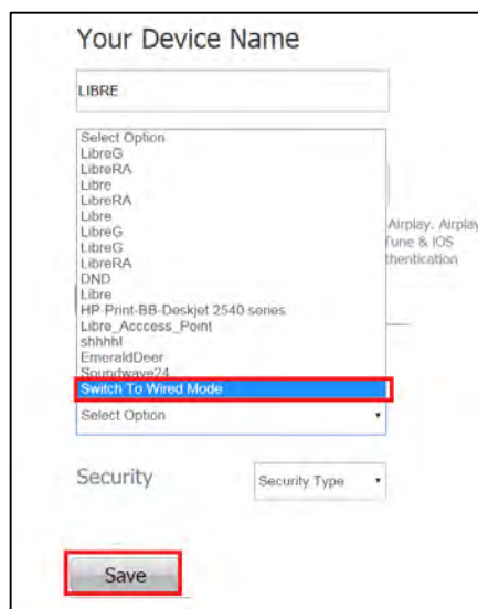
Figure 6.11-1: Switch to Wired Mode
