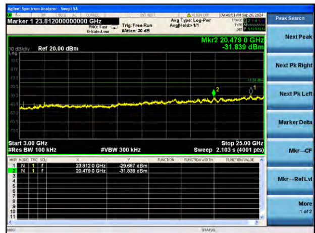
GFSK LOW CHANNEL, SPURIOUS 3 GHz ~ 25 GHz
