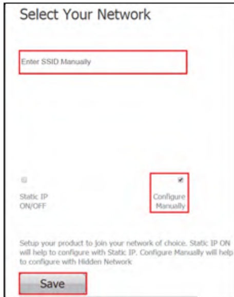
Figure 6.2.3-1: Configure Network Manually
