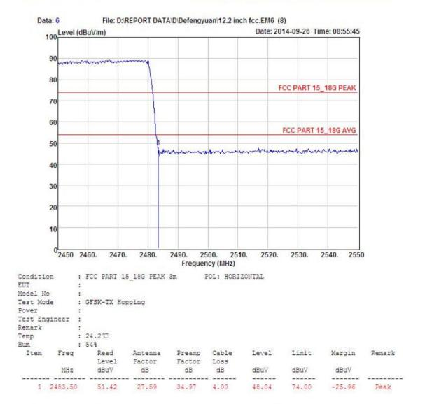
Remark: Level = Read Level + Antenna Factor - Preamp Factor + Cable Loss
