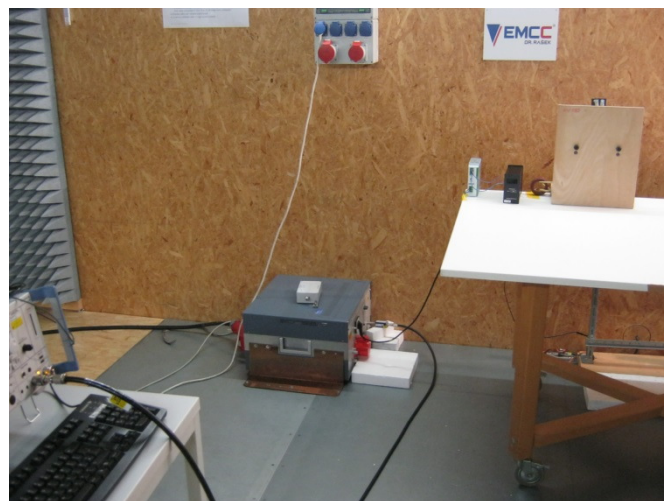
Conducted emissions measurement 150 kHz – 30 MHz
