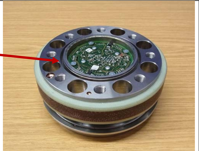
The rotor includes 4 PCB*
