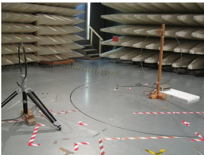
Correlation measurement with single turn loop antenna and signal generator in SAC, 3m distance
