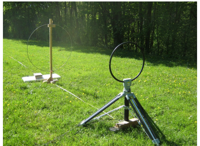
Correlation measurement with single turn loop antenna and signal generator at open area test site, 3m distance
