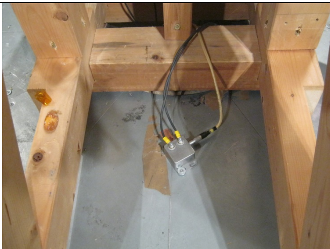
Detail on Axon stator unit connected to stator and connection cable to Axon system control unit
