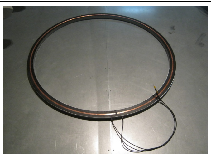
Detail on stator antenna with connection cables
