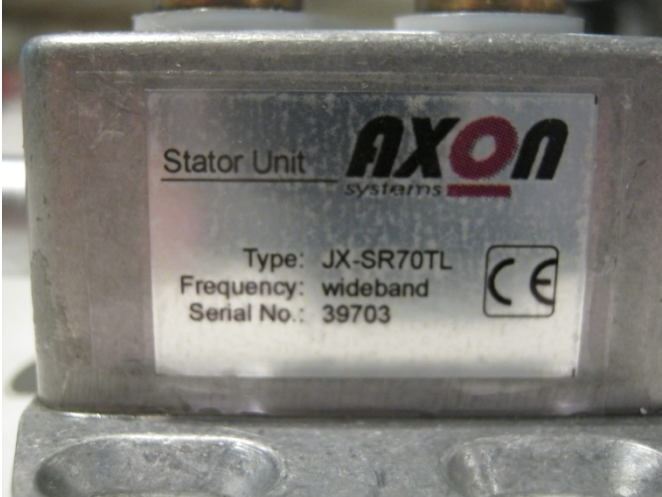
Photograph 2.3-5: Label of the Axon Stator Unit used for the antenna connection
