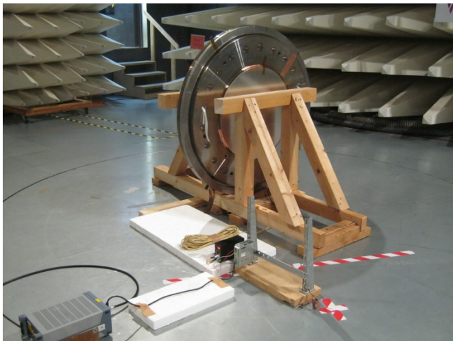
Conducted emissions measurement 150 kHz – 30 MHz
