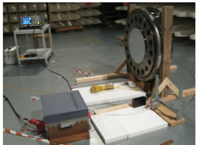
Conducted emissions measurement 150 kHz – 30 MHz
