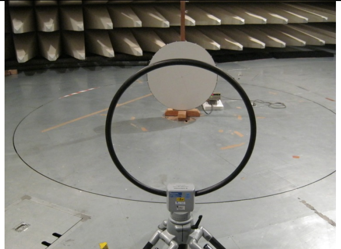
H field measurement in SAC at 3 m distance
