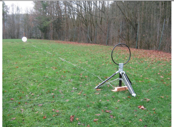
H field measurement at open field site at 30 m distance
