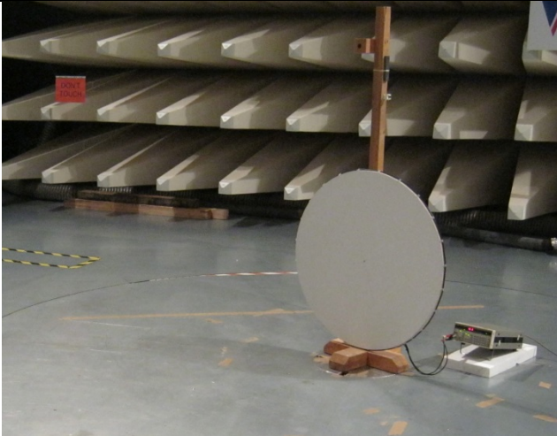
Single turn loop antenna with signal generator
